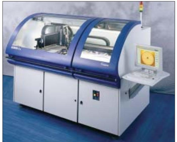
*Photo 1. An automated platform for polishing cleaning and inspection for connectors, includes process technology and supporting servo motion control and software for adaptive process control.*
